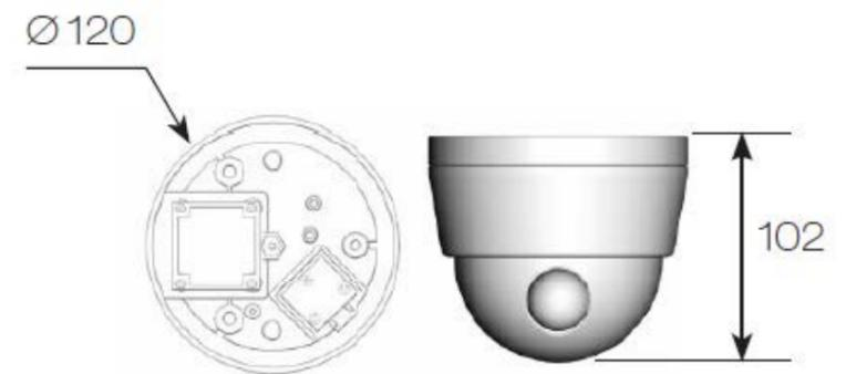
Fixed dome LR2122 in the L series is featuring built-in Sense up+ technology to deliver stunning video in low-light conditions. Utilizing intelligent image signal processing, 2D WDR function, AGC control, and 3D Noise Reduction, the combination successfully delivers the ultimate low-light image without motion blur. Support with PoE, privacy mask, White balance, and minimum illumination 0.15 Lux at F 1.6 Low Light Mode or 0.18 Lux at F1.8 Low Light Mode.
