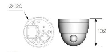
Diagram of mounting holes (unit in mm):
