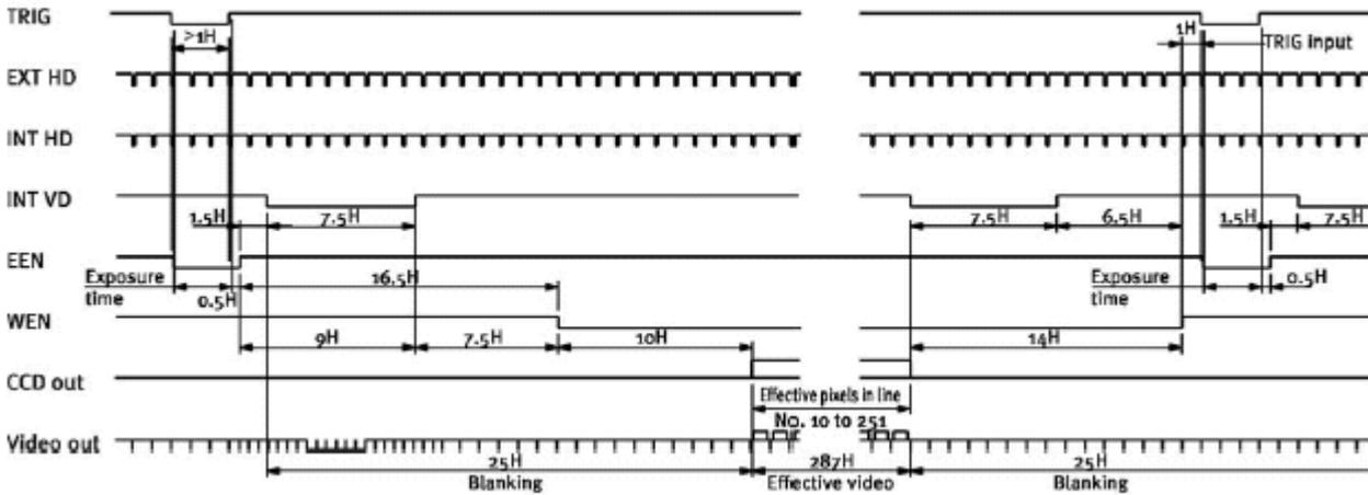
Note: • Do not input external VD signal at Pin No. 7 of the 12-pin Hirose connector, as it may disturb the external trigger function.
