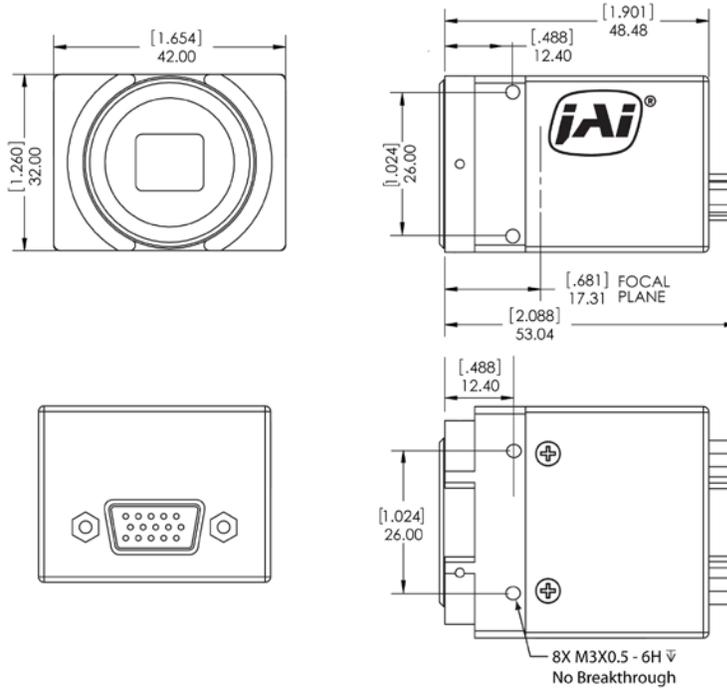
**Caution:** When mounting the camera to any fixture, do not use screws that extend more than 5 mm into the camera housing to avoid possible damage to the internal circuitry. For attaching the tripod mounting plate, only the supplied screws should be used.
