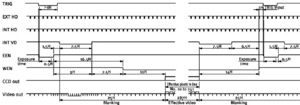
Note: • The duration of the external trigger pulse must be greater than 1H. It is recommended to make this longer, typically 9H.
