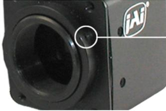
Loosen the three 2mm screws around the perimeter of the C-mount lens collar to adjust the back focus.
