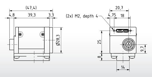
Dimensions: mm Tolerances: DIN ISO 2768m
