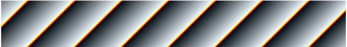
Fig. 63: Static Image of Test Pattern 4 with Spatial Correction Set to +8
