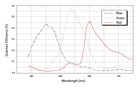
The spectral response curve excludes lens characteristics, light source characteristics, and IR cut filter characteristics.
