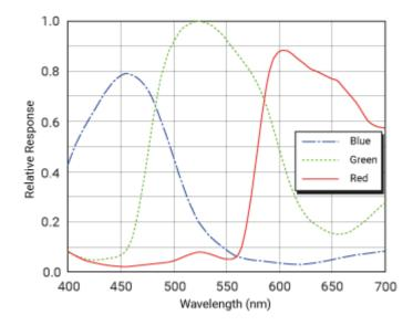
The spectral response curves exclude lens characteristics, light source characteristics, and IR cut filter characteristics.
