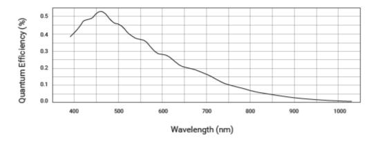
The spectral response curve excludes lens characteristics and light source characteristics.
