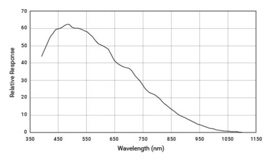
The spectral response curve excludes lens characteristics and light source characteristics.
