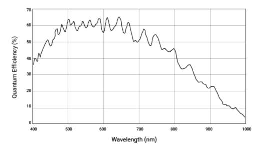
The spectral response curve excludes lens characteristics and light source characteristics.
