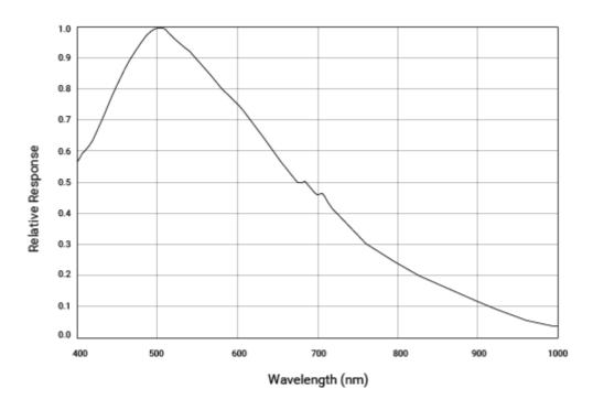
The spectral response curve excludes lens characteristics and light source characteristics.
