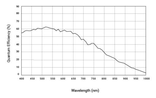
The spectral response curve excludes lens characteristics and light source characteristics.
