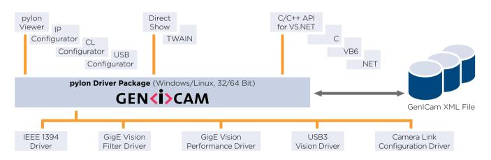
The internal architecture of the pylon driver package is based on GenlCam Technology, which offers you easy access to the newest camera models and the latest features. Changes to an existing camera device in your application essentially become a plug-andplay process.
