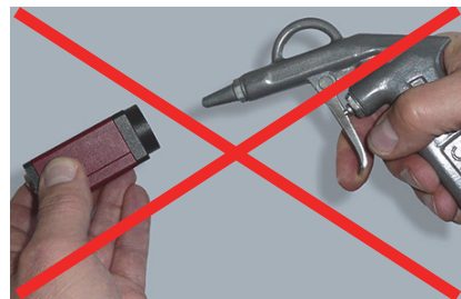
Figure 6: Do not use compressed air
